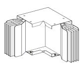
Flat elbow, Canalis KTA, aluminium, 1600A, 3L+N+PER (Cu), high lcw, N1, 2 made to measure branches, right angle
