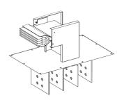
Flat elbow feed unit, Canalis KTA, aluminium, 800A, 3L+PE, made to measure dimensions, neutral N3, white RAL9001
