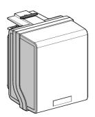
Tap off unit, Canalis KS 100A to 1000A, with fuse holder, 16A, NZ fuses not supplied, 3L+N+PE, IP55, RAL9001
