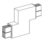
Edgewise zed unit, Canalis KRC, copper, 1000A, 3L, made to measure, grey RAL7030
