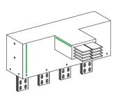
Flat elbow feed unit, Canalis KRC, copper, 1000A, 3L, made to measure dimensions, flat connection pads, grey RAL7030
