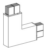
Edgewise elbow, Canalis KRA, aluminium, 5000A, 3L+N+PE, made to measure length 0.5-1m, grey RAL7030
