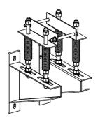
Vertical wall spring support, Canalis KRA, vertical busbar trunking (aluminium), 4000A, 5 conductors busbar
