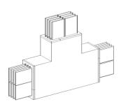
Edgewise tee, Canalis KRA, aluminium, 4000A, 3L+N+PE, made to measure length 0.5-1m, grey RAL7030
