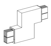
Edgewise zed unit, Canalis KRA, aluminium, 2000A, 3L+N°PE, made to measure, grey RAL7030
