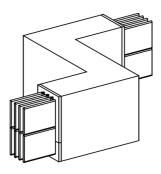
Flat zed unit, Canalis KRA, aluminium, 1600A, 3L+N°PE, made to measure, grey RAL7030
