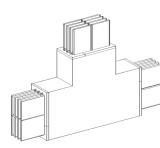
Edgewise tee, Canalis KRA, aluminium, 1600A, 3L+N/3L+PE/ 3L+PEN, made to measure length 0.35-1.15m, grey RAL7030
