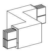
Flat zed unit, Canalis KRA, aluminium, 1000A, 3L+N/3L+PE/ 3L+PEN, made to measure, grey RAL7030
