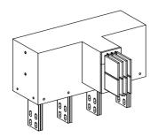
Edgewise elbow feed unit, Canalis KRA, aluminium, 800A, 3L+N/ 3L+PE/3L+PEN, made to measure dimensions, grey RAL7030
