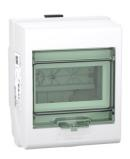
Tap off unit, Canalis KN, for modular devices, 32A, 3L+N+PE, up to 5 modules of 18mm, IP55
