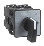
Cam stepping switch, Harmony K, multifixing, plastic,1 pole, 4 steps, position 0, 45°,12A, 45x45mm, metallic legend, 35mm black handle
