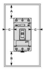
Toggle-type, rotary handle-type: identical clearance values
