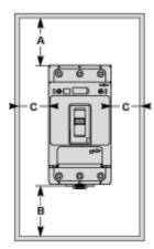
Toggle-type, rotary handle-type: identical clearance values.
