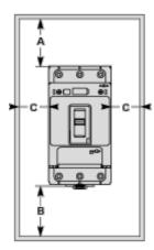
Toggle-type, rotary handle-type: identical clearance values
