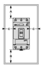
Toggle-type, rotary handle-type: identical clearance values.
