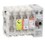
Switch disconnector fuse, TeSys GS, 4P, 50A, fuse type NFC, size 14x51mm
