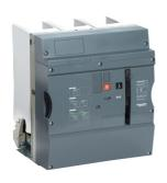
MV vacuum circuit breaker, EasyPact EXE, basic function, 12kV, 1250A, 20kA 3s, 185mm, IEC
