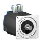
AC servo motor BSH, Lexium 05, 14.9N.m, 1500rpm, untapped shaft, with brake, IP50
