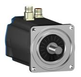
AC servo motor BSH, Lexium 05, 9.31N.m, 1500rpm, keyed shaft, with brake, IP50
