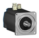
servo motor BSH, Lexium 05, 9.31N.m, 1500rpm, 100mm, untapped shaft, Sincos single turn, with brake, IP50, straight
