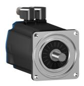
servo motor BSH, Lexium 05, 5.5N.m, 4000rpm, 100mm, keyed shaft, Sincos multi turn, without brake, IP65
