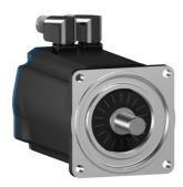
servo motor BSH, Lexium 05, 3.4N.m, 2500rpm, 100mm, keyed shaft, Sincos multi turn, without brake, IP50
