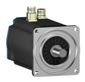
servo motor BSH, Lexium 05, 3.4N.m, 2500rpm, 100mm, keyed shaft, Sincos multi turn, without brake, IP50, straight
