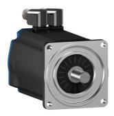
servo motor BSH, Lexium 05, 3.4N.m, 2500rpm, 100mm, keyed shaft, Sincos single turn, with brake, IP50
