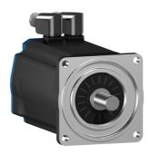
servo motor BSH, Lexium 05, 3.4N.m, 2500rpm, 100mm, untapped shaft, Sincos multi turn, with brake, IP50
