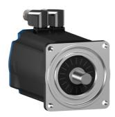
servo motor BSH, Lexium 05, 3.39N.m, 4000rpm, 100mm, keyed shaft, Sincos single turn, without brake, IP65
