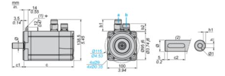
a: Power supply for servo motor brake
