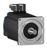
servo motor BSH, Lexium 05, 2.7N.m, 3000rpm, 100mm, keyed shaft, Sincos multi turn, with brake, IP50
