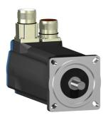
servo motor BSH, Lexium 05, 2.2N.m, 3000rpm, 70mm, keyed shaft, Sincos single turn, with brake, IP50, straight
