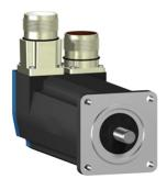
servo motor BSH, Lexium 05, 1.3N.m, 3000rpm, 55mm, keyed shaft, Sincos single turn, without brake, IP50, straight
