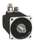
servo motor BMH, Lexium 32, 3.3Nm, 6000rpm, untapped shaft, with brake, IP54, 128 multiturn encoder, straight
