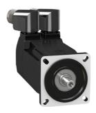
servo motor BMH, Lexium 32, 3.4Nm, 8000rpm, untapped shaft, with brake, IP65, IP67, 16 multiturn encoder, 3 phases
