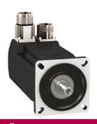
servo motor BMH, Lexium 32, 2.5Nm, 8000rpm, untapped shaft, without brake, IP65, IP67, 16 multiturn encoder, straight
