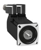
servo motor BMH, Lexium 32, 2.5Nm, 8000rpm, keyed shaft, without brake, IP54, 16 multiturn encoder, 3 phases
