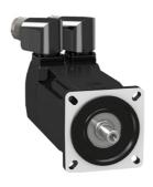
servo motor BMH, Lexium 32, 1.4Nm, 8000rpm, untapped shaft, with brake, IP65, IP67, 16 multiturn encoder
