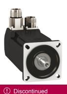
servo motor BMH, Lexium 32, 1.2Nm, 8000rpm, keyed shaft, without brake, IP65, IP67, 16bit encoder, straight
