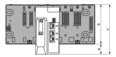
a: additional space below the rack to accommodate the height of the CPU. For an X Bus rack, the value is 30.9 mm (1.217 in.); for an Ethernet rack, the value is 29.49 mm (1.161 in.).
