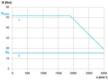
Servo Motor with LXM28AU45 ••• Servo Drive
