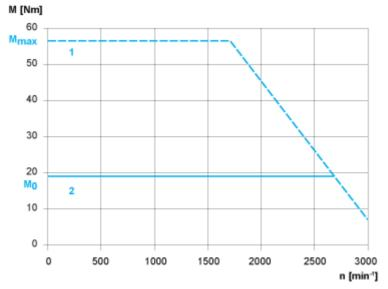
Servo Motor with LXM28AU30 ••• Servo Drive
