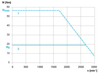
Servo Motor with LXM28AU30 ••• Servo Drive
