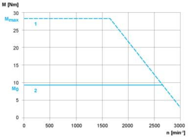
Servo Motor with LXM28AU20 ••• Servo Drive
