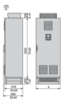
Standard Floor-Standing Enclosure + Additional Enclosures, According to the Configuration
