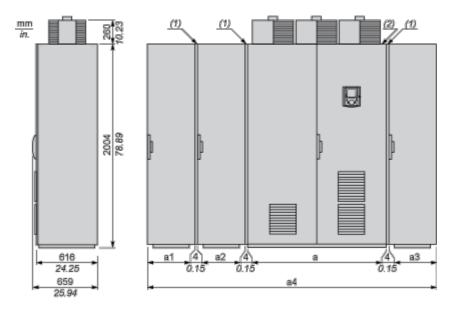
$(1) \qquad \mbox{Seal. For each floor-standing enclosure added, allow a 4 mm/0.15 in. space for the seal.}$
