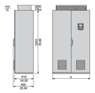
Standard Compact Floor-Standing Enclosure + Additional Floor-Standing Enclosures, According to the Configuration
