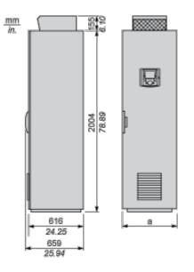
Standard Compact Floor-Standing Enclosure + Additional Floor-Standing Enclosures, According to the Configuration
