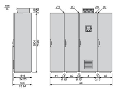
(1) Seal. For each floor-standing enclosure added, allow a 4 mm/0.15 in. space for the seal.
